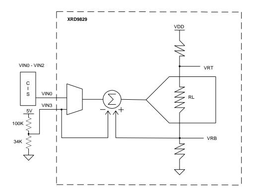
Figure 7. Simplified Block Diagram Showing Global Offset Adjustment by XRD9829
